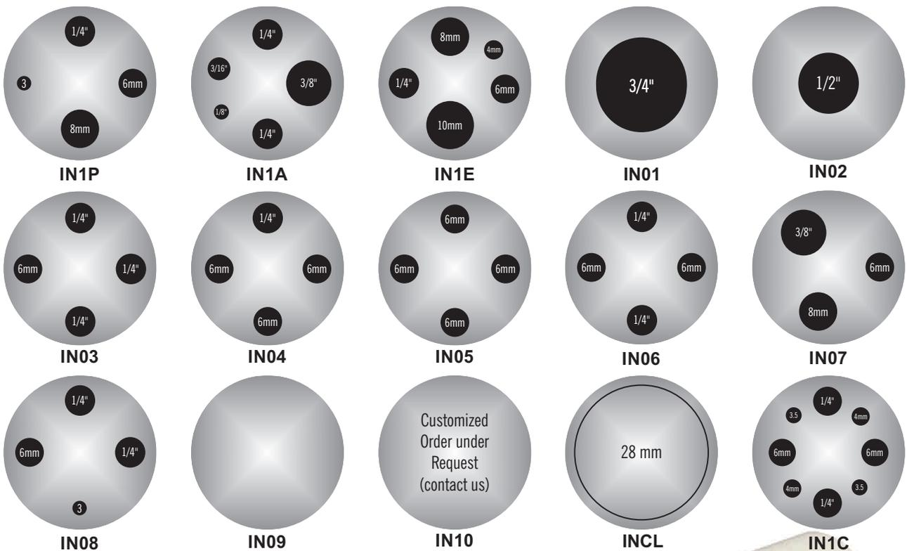
The use of unappropriated inserts and wrong material can provide unexpected results or cause damages to your unit. In case you need a customized insert, consult your distributor or the factory. Presys can provide custom inserts with minimum 3 mm separation between holes.
