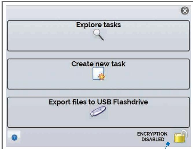
Communication with your calibration software applications such as ISOPLAN® are encrypted to assure the integrity of your calibration data in accordance with 21 CFR Part 11. When activated by the administrator, the XML data file with calibration information will be encrypted.
